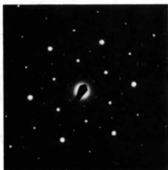
Fig. 4. Diffraction pattern at a temperature > 773 K, (0001)^* section; weak pseudospots of \frac{1}{2}\{10\bar{1}0\} type appear.
