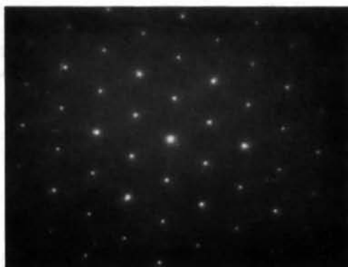
Fig. 6. Diffraction patterns from the (0001)^* section where superlattice spots are absent.
